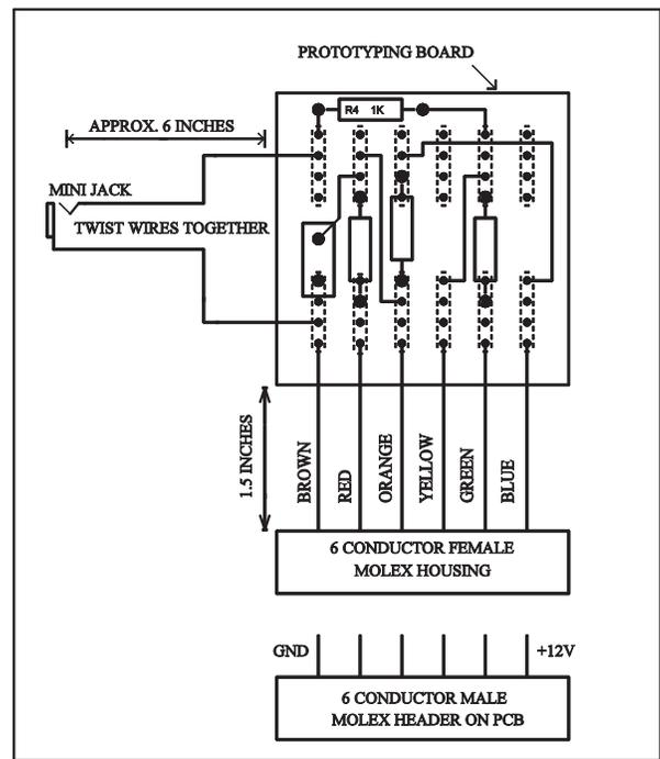
Figure 9b - Component Layout of Volume CV Board
