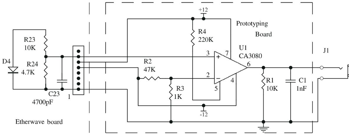
Figure 7 - Output Amplifier for Tuner
