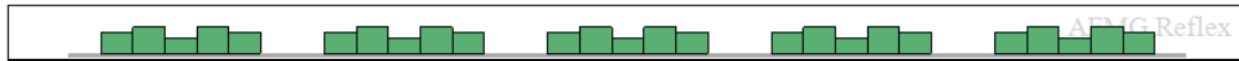
Depth Profile of Diffuser Array with No Profiled Modulation 1 (Simulation View in AFMG Reflex)
