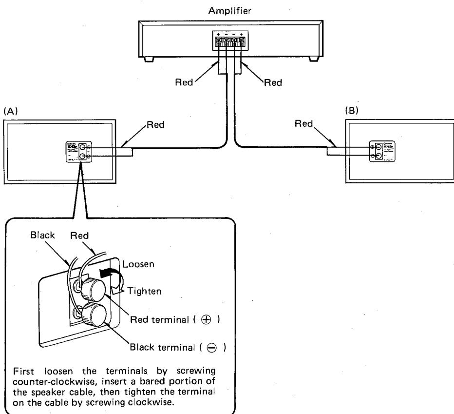
First loosen the terminals by screwing counter-clockwise, insert a bared portion of the speaker cable, then tighten the terminal on the cable by screwing clockwise.
